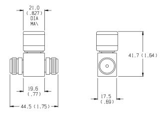
NOTE: All dimensions are given in mm (inches) and are maximum, unless otherwise specified.
